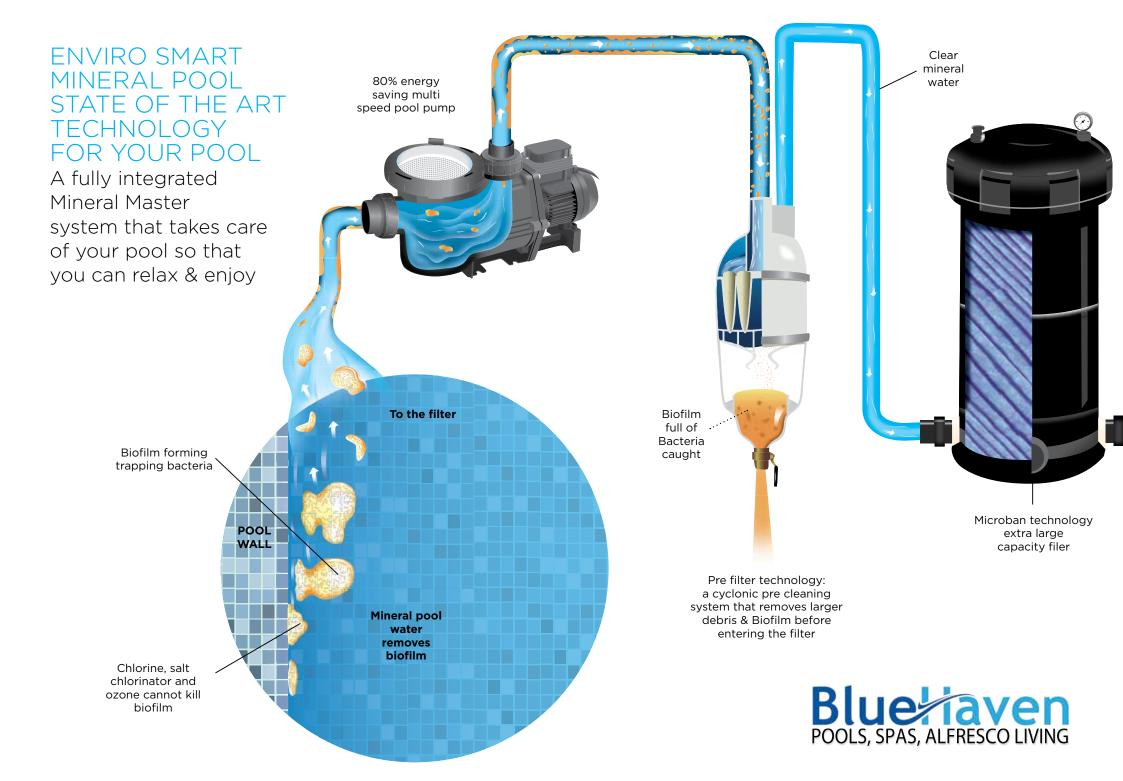
Mineral converter designed to convert Mineral Pool Blend in to the required sanitisation to keep healthy soft crystal clear water
